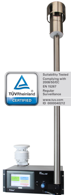
Certified fine dust measurement device Fidas 200, TÜV Rheinland certified, TÜV cer
