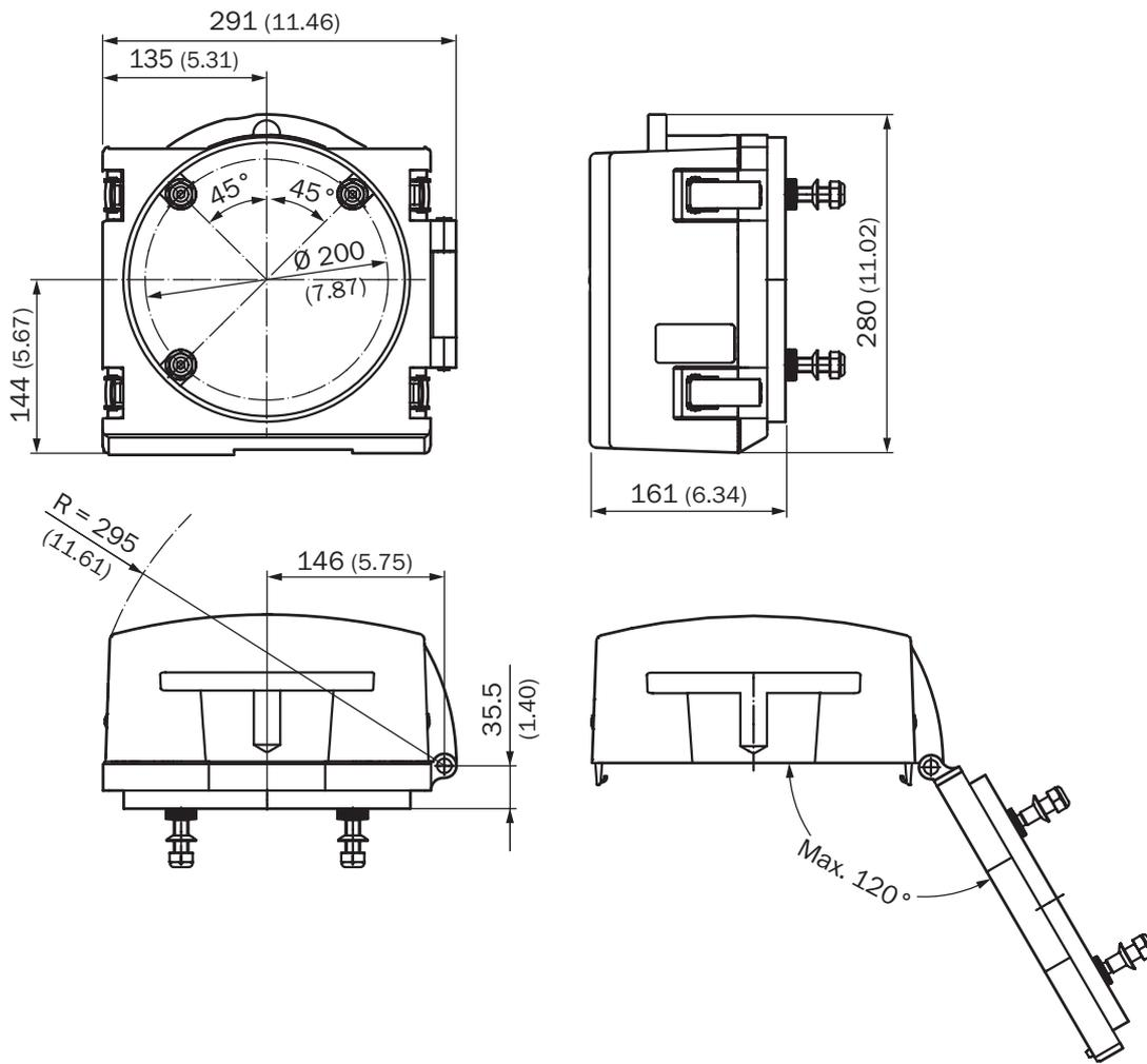
Connection unit; standard version (dimensions in mm (inch))
