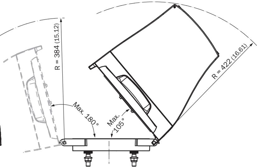
Sender/receiver unit; Ex-version (dimensions in mm (inch))
