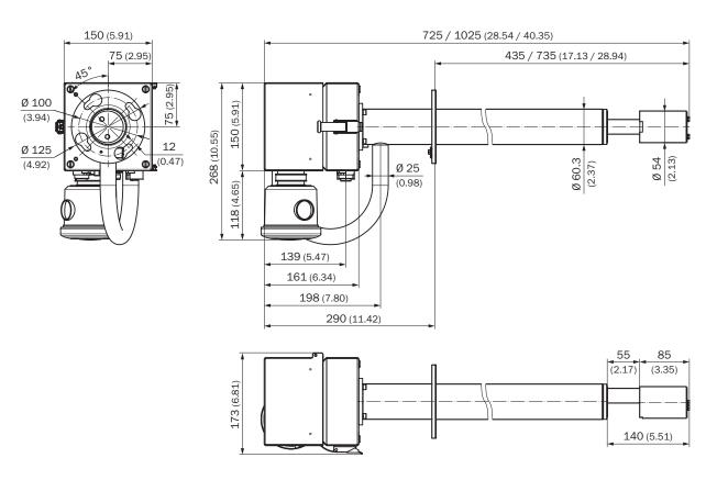
Sender/receiver unit DHSP30, 1" thread, nominal length = 180 mm (dimensions in mm (inch)
