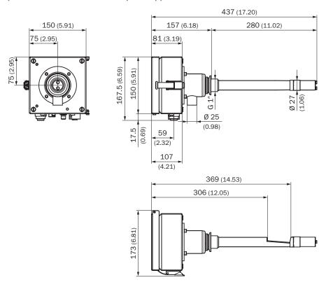
Sender/receiver unit DHSP30, TriClamp, nominal length = 280 mm, with integrated purge air unit (dimensions in mm (inch))
