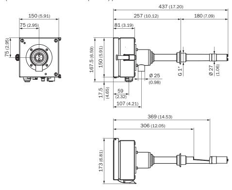
Sender/receiver unit DHSP30, TriClamp, nominal length = 180 mm, with integrated purge air unit (dimensions in mm (inch))
