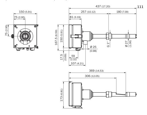
Sender/receiver unit DHSP30, 1" thread, nominal length = 180 mm, with integrated purge air unit (dimensions in mm (inch))
