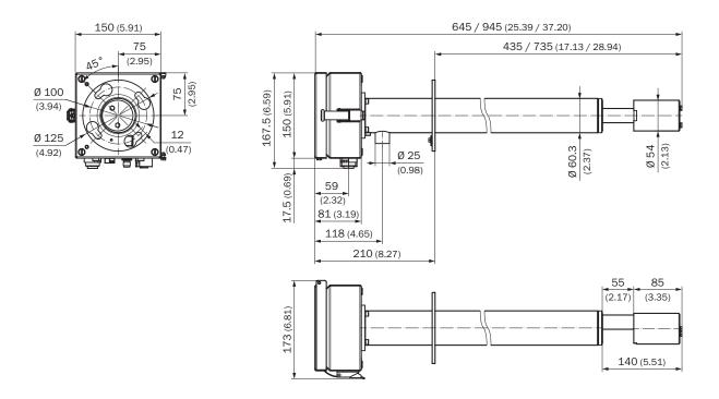
Sender/receiver unit DHSP30, flange version, with integrated purge air unit (dimensions in mm (inch))
