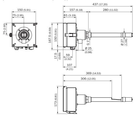
Sender/receiver unit DHSP30, 1" thread, nominal length = 280 mm, with integrated purge air unit(dimensions in mm (inch))
