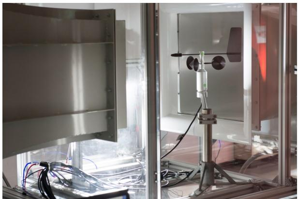
► *LSI LASTEM is an ISO17025 accredited laboratory for air speed measurements. All sensors manufactured are tested inside this laboratory. LSI LASTEM provides Test report for any sensor supplied and on request, ISO17025 or ISO9001 calibration certificates (see Accessories list).*
