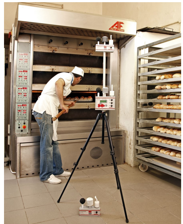
Three levels WBGT on the same vertical
