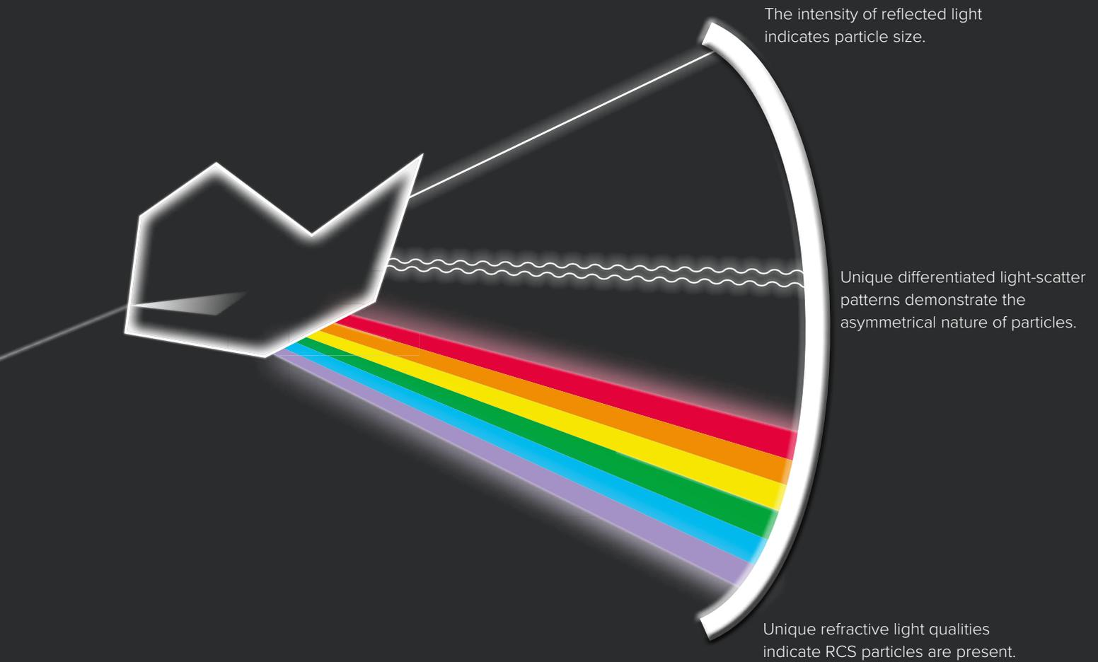
Our Breathe<sup>+</sup> high-speed scatter/sizing/crystallinity detection algorithm processes the results in real time and triggers a triple-voting system that positively identifies and distinguishes harmful silica content.
