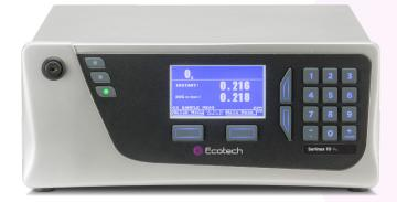
The Serinus® 10 Ozone ( $O_3$ ) analyser delivers precise and reliable performance at excellent value. It uses proven non-dispersive ultraviolet (UV) absorption technology to measure  $O_3$  in ambient air (LDL < 0.5 ppb, range 0 to 20 ppm).
