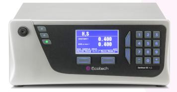
The Serinus® 55 Hydrogen Sulfide (H<sub>2</sub>S) analyser delivers precise and reliable performance at excellent value. It uses proven UV fluorescent radiation technology and an internal thermal catalytic converter to measure H<sub>2</sub>S in ambient air (LDL < 0.3 ppb, range 0-2 ppm).
