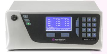
The Serinus® 44 analyser delivers precise and reliable performance at excellent value. It uses proven chemiluminescence technology and an external thermal catalytic converter to measure NO, NO<sub>2</sub>, NO<sub>x</sub> and NH<sub>3</sub> in ambient air (LDL < 0.4 ppb, range 0 to 20 ppm).
