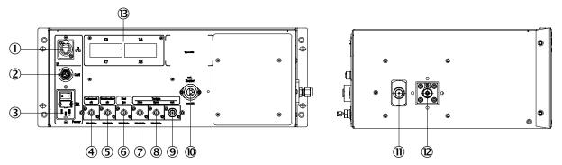
GMS810 FIDOR and GMS811 FIDOR: sample gas inlet on the side
