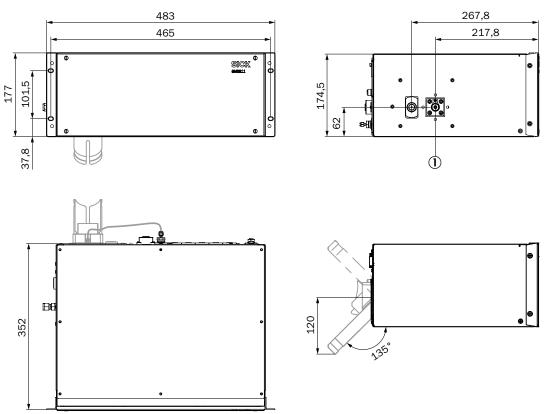
0 On the GMS811 FIDOR, the sample gas inlet can be located on the side or on the rear (shown in light grey).
