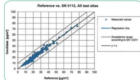
Reference equivalence function for PM<sub>10</sub> for Fidas® 200 and Fidas® 200 S
