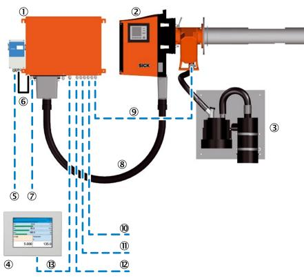
1 Connection unit with Ex-p controller for Zone 1 (2G) and Zone 2 (3G)
