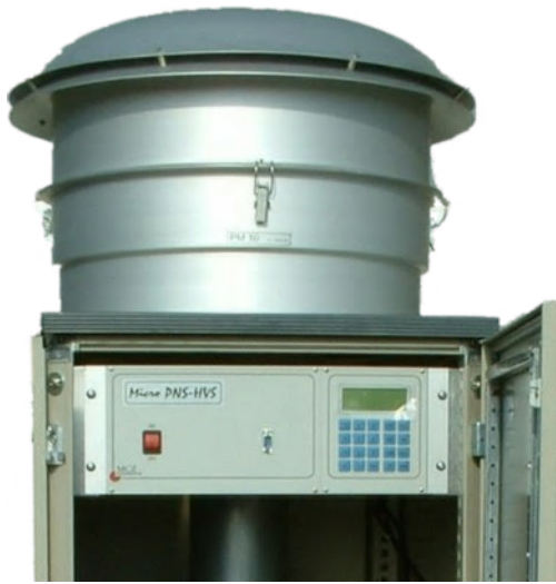
MicroPNS control unit with PM 10 sampling inlet for 68m 3 /h cutpoint
