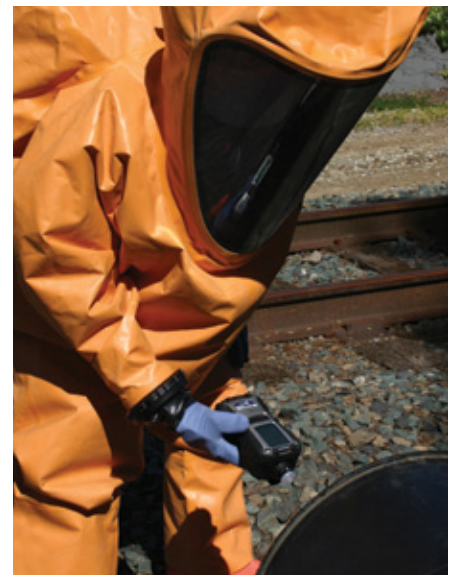
CBRN detection with the MultiRAE Pro
