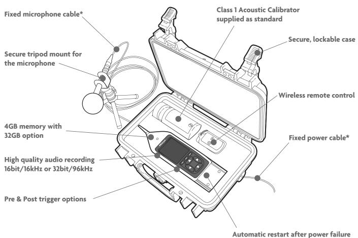
\*Cables can be removed when case is open
